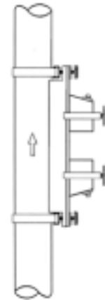
Fig. 4.9: Recommended ultrasonic converter positioning in vertical pipes
